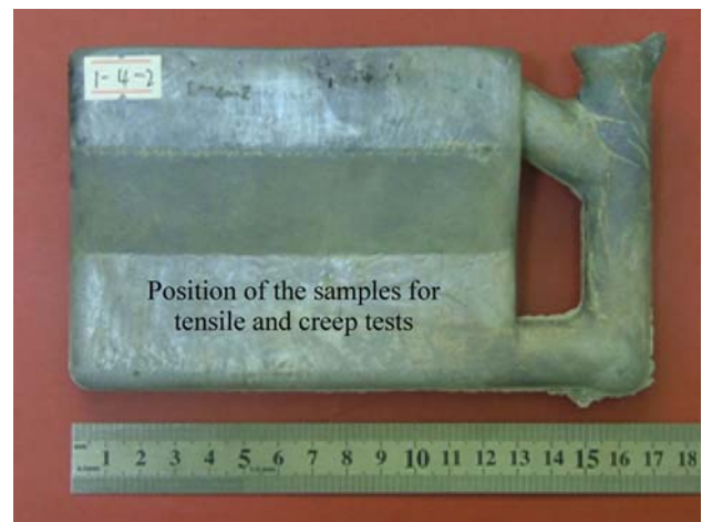
Fig. 1 Image for the pouring casting of the experimental alloys
